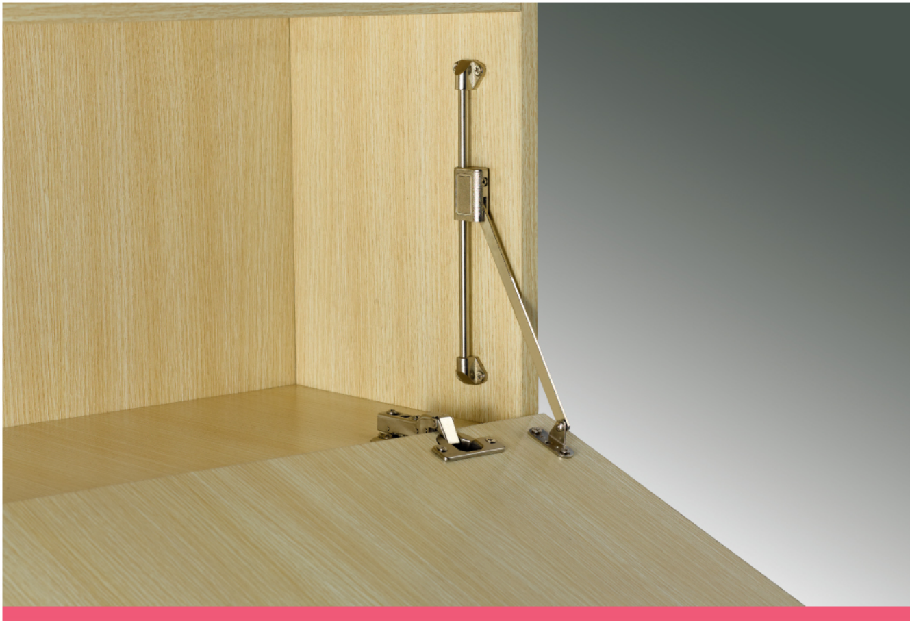
Multifunctional Flap Support(Down Lifting) Material: Iron Finsih: Zinc plated Available for : Down-turning wooden door and aluminu-frame door Function: Supporting cabinet doors International advanced spray-paint technology
